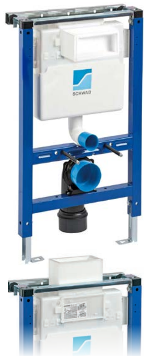
Duplo 187 Frame Front or Top Activation £240.00 500 x 820-1020 x 150-210
